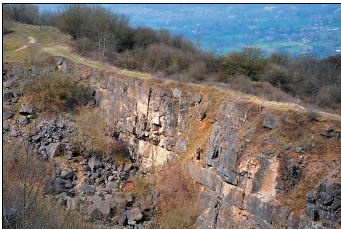
Figure 4. The eastern face, about 15 m high, of the Masson Hill open pit; the Matlock Upper Lava is at the top right corner of the face.
