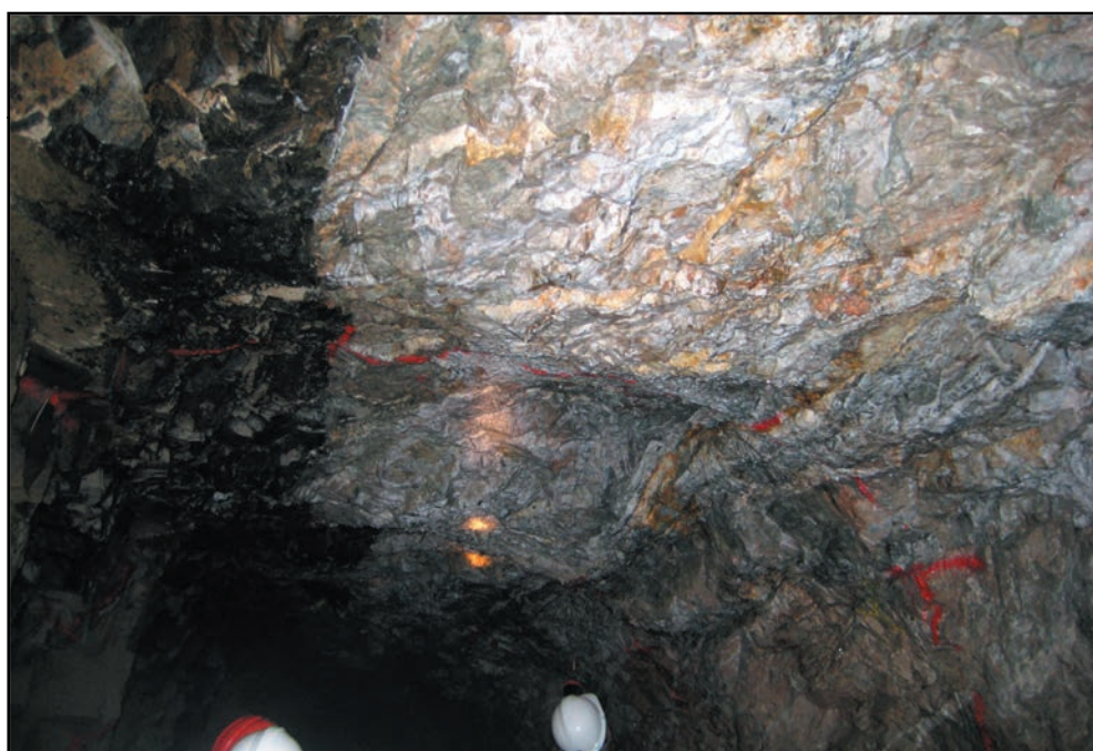
Figure 18. Mineralised quartz vein against a dolerite dyke in the roof of the Cononish adit (photo: Gus Gunn).
