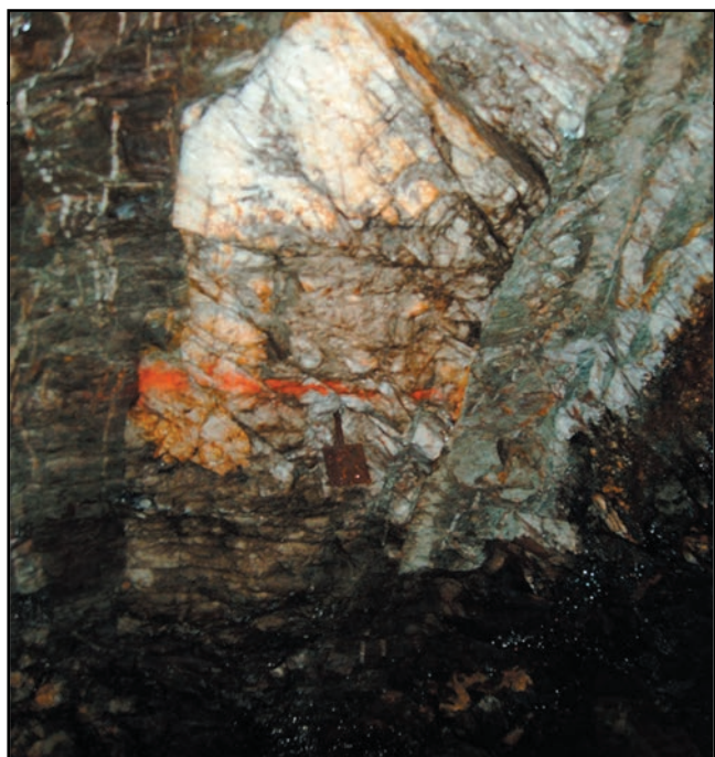
Figure 17. Gold-bearing quartz-sulphide vein along the roof of the 1985 adit in the Curraghinalt prospect.
