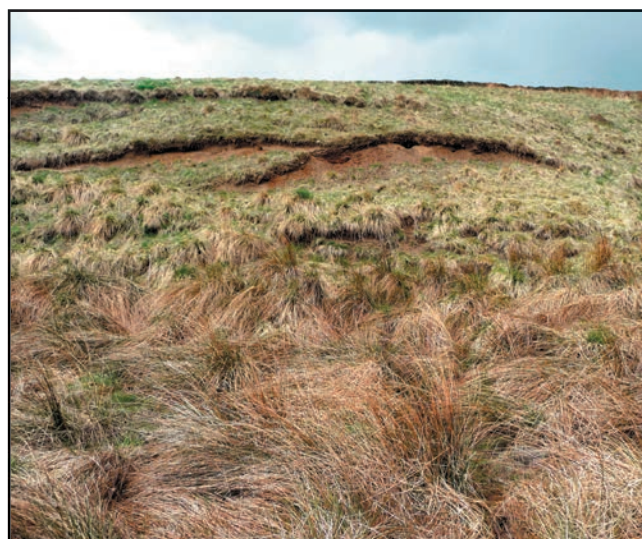
Figure 8. Small back scars above and behind shallow planar failures within the regolith.
