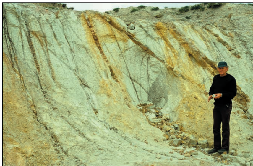
Figure 11 (Left). Kaolinised granite streaked with dark mineral veins exposed in the small open pit in the orebody of tungsten and tin at Hemerdon.
